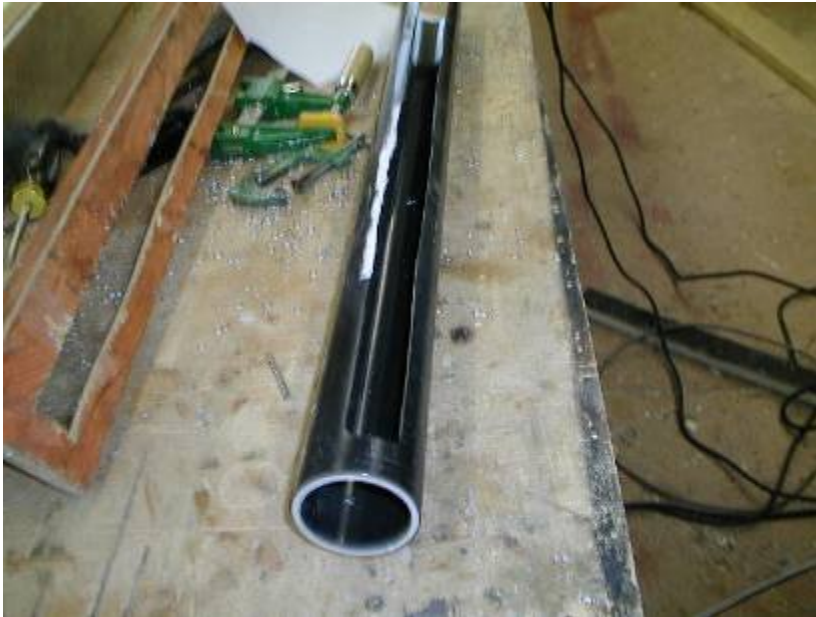
Completed Drain Tube for one Collector.
