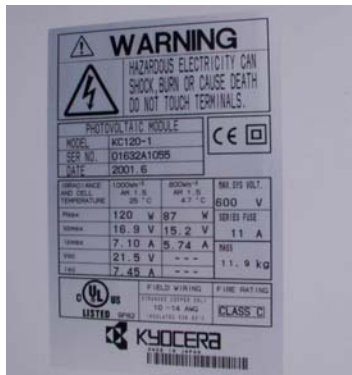
Figure 1 PV Module Listing Label
