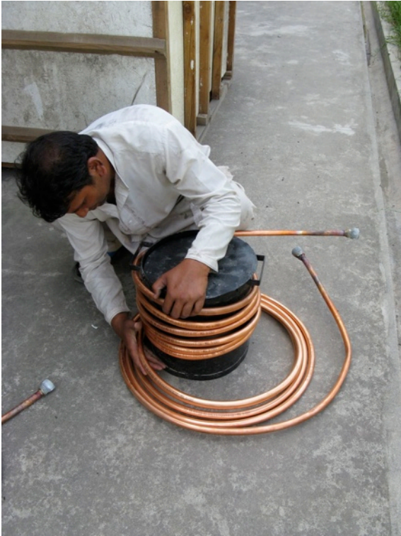
Heat exchanger winding.
