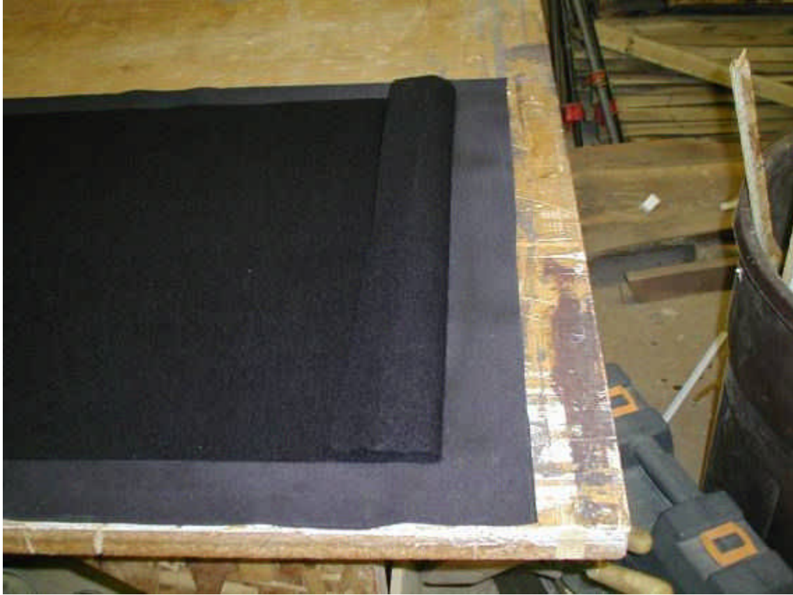
Top of the Trickle Down Matt "TDM". The felt is cut long so that it can be folded back down over the trickle tube.
