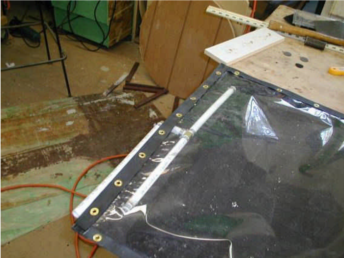
The extra length of felt is folded up over the trickle tube. Just showing how the tube is installed in this pic.
