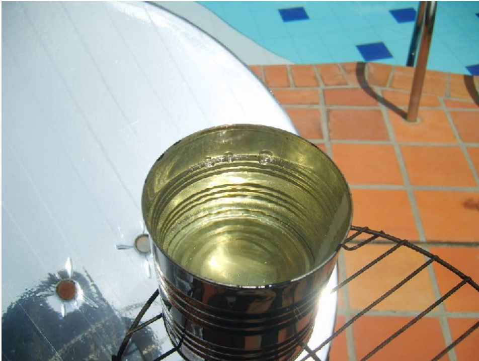
Figure 8. A real boil in just over 20 minutes, having put a cap over the can just after the first bubbles appeared.
