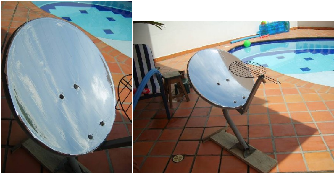
Figure 4. The dish with the new reflective surface and mounted on its original structure.
