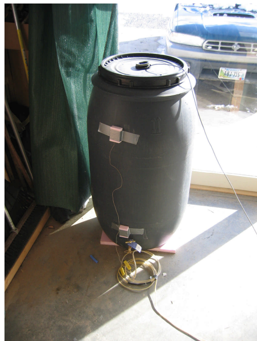
Testing water barrels for thermal mass.
