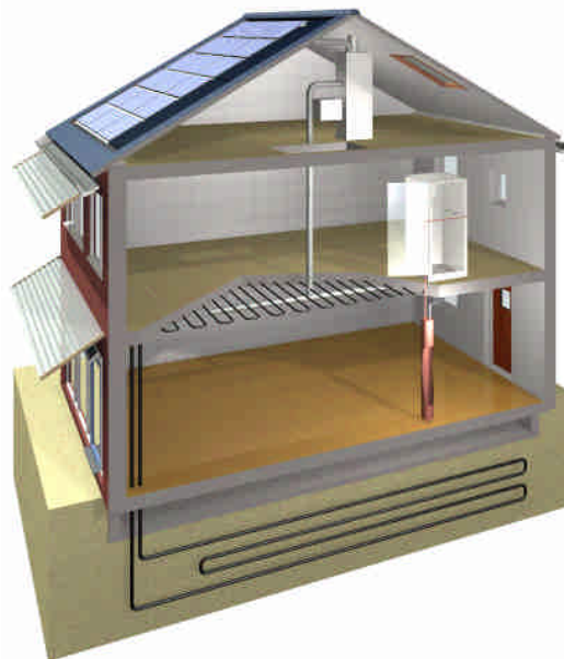
Figure 2: The system configuration in the A-house. The heat pump boiler is located in the attic.
