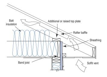
A raised top plate increases the height for insulation and ventilation at the eaves.
