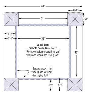
Cut out and discard four corners of fiberglass duct board
