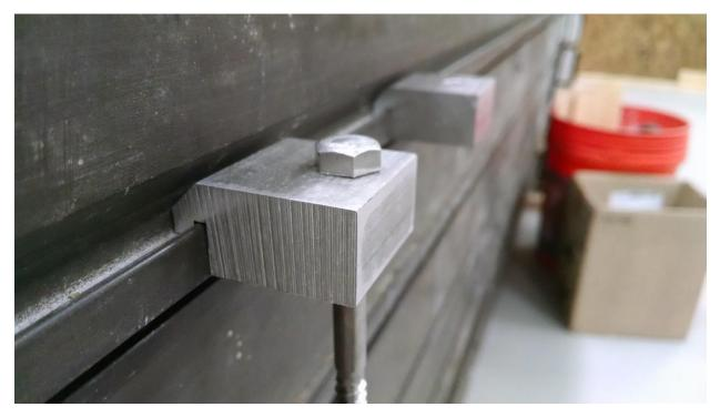
Custom made mounting brackets with a stainless-steel lag screw.
