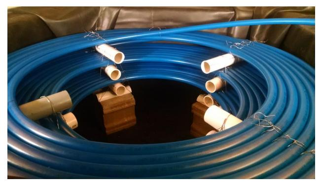
Finished Heat Exchanger coil.
