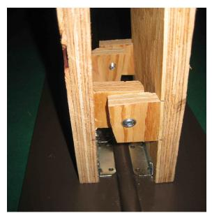
Illustration 7: Fin clamping tool in action.
