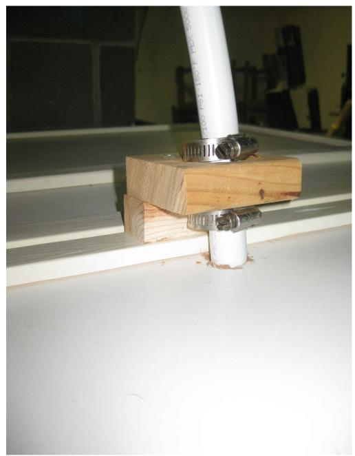
Illustration 7: close-up showing bracket and clamps holding return line in place at the tank. These can be easily adjusted or loosened if it is necessary to remove tube for service.
