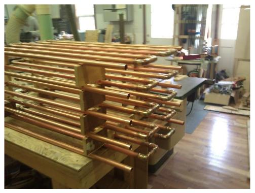
Here is the completed heat exchanger ready to be dropped into the tank (suspended actually, it sits in the top half of the tank).
