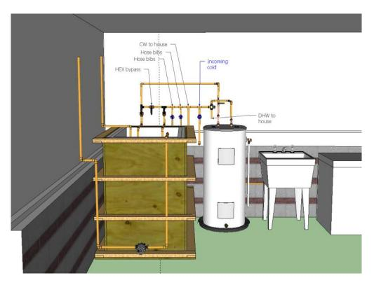
The tank is  $28''w \times 44'' \times 46''d$  inside dimension. In the final version, the framing is vertical between the upper and lower bands. The lower band is attached to a  $\frac{3}{4}''$  PT plywood base for lateral strength.
