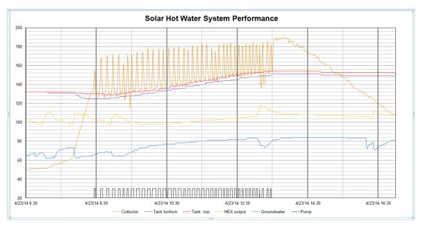
The current settings on Max are On at  $18^{\circ}$ F differential and Off at  $5^{\circ}$ F differential. The seemingly excessive cycling of the pump on the  $22^{nd}$  would seem to indicate that the Off differential might need to be reduced to  $2^{\circ}$ F or  $3^{\circ}$ F.
