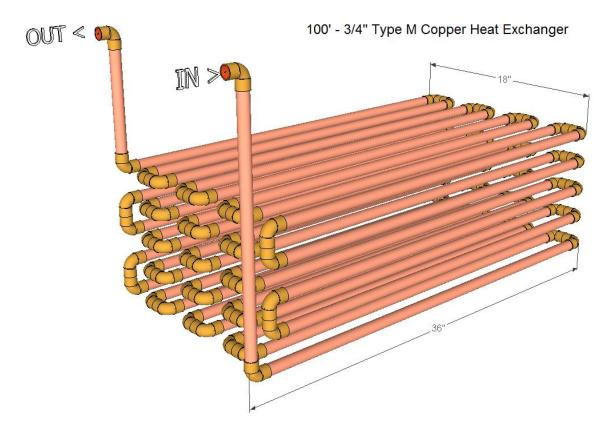
Because of the cost of soft copper tubing, I elected to make my heat exchanger from hard copper pipe, as I wanted a better thermal transfer property than the PEX provides. The process started by building a jig for making the "level" sub-assemblies of the HEX:
