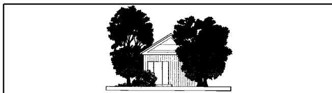
Figure 12. For air-conditioned homes, low-branching trees placed by windows provide protection against air movement.
