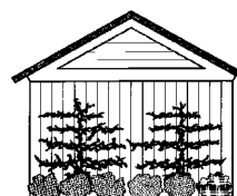
Figure 6. Espaliered shrubs can insulate a wall from heat build-up.
