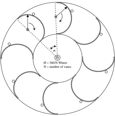
the direction of the proposed slots such that when the disks are assembled, the slots will correspond to one another.
