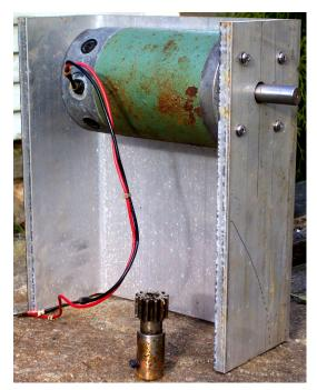
again by 3 to 1 in order to reach an appropriate speed of 1000 rpm for my particular generator. For this I'm using roller chain and sprockets (U.S. TSUBAKI 40B9F-5/8 and 40B28F-5/8) on a 5/8 inch axle to be installed in the chassis shown.
