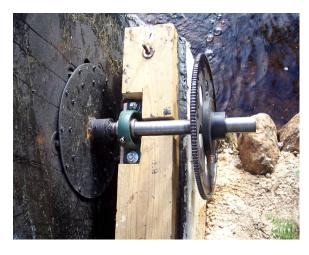
wheel after locating the center of rotation as best as I could with a tape measure. It is truly important that this be done accurately since any error will result in a multi-axis wobble and reduced clearance to the sluice.
