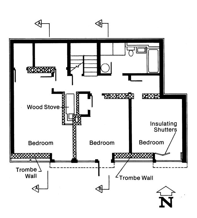
terior walls. These surfaces function as solar absorbers, turning the sunlight into heat. The heat is conducted into the interior mass of the floor and walls, where it is stored.
