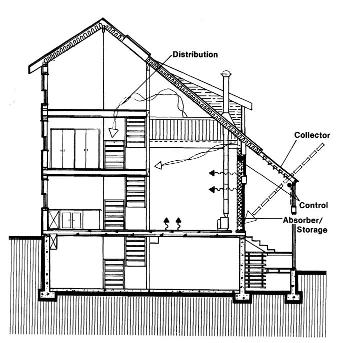
control the heat gain or to store it. However, by providing some daytime heating, it allows the other two systems to store a larger amount of heat for nighttime use.
