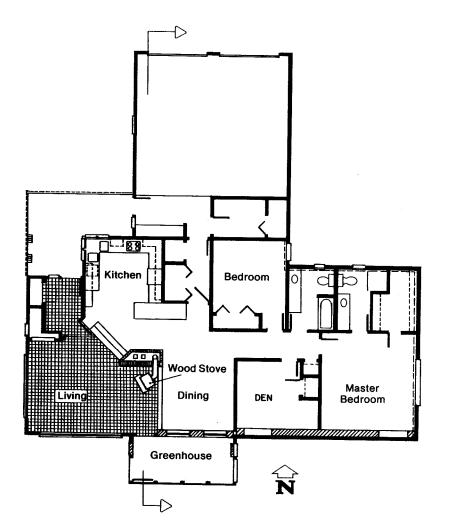
In colder weather, hot air that accumulates at the cathedral ceiling is drawn down the brick chimney enclosure by a small fan and vented onto the kitchen floor. This air is heated further when the stove is being used because the sealed flue within the chimney heats room air.
