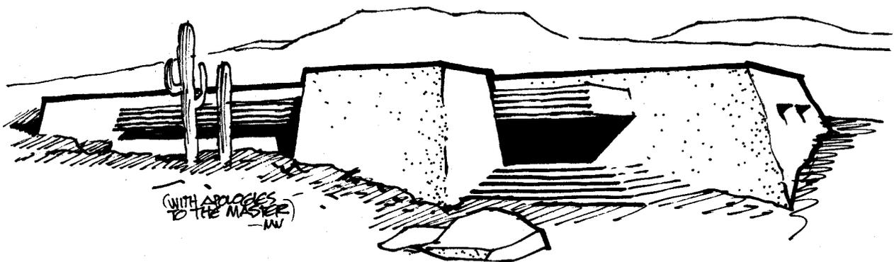
In arid climates, earth contact can provide pleasant relief from hot weather and does not have associated moisture problems since humidity is often encouraged. Earth pipes can be perforated to increase humidification of the air by the ground.
