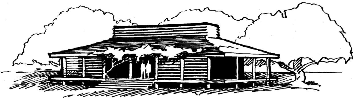
A partial solution to this dilemma is a house that is both well insulated and well shaded. Windows should be double-glazed. For removing the winter chill, one third to one half of the total window area should face south. Properly designed houses will require little if any other heat in most winter climates of less than 3000 degree days per year.
