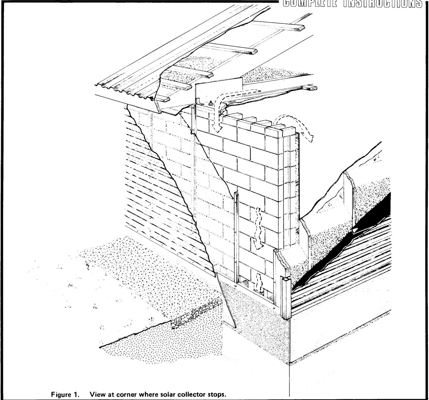
Figure 1. View at corner where solar collector stops.
