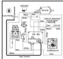
NOTE: The ON/OFF switch, located in line with the gas valve, is not used when a combination circuit breaker and ON/OFF switch is used.
