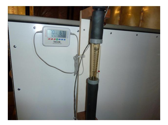
Flow meter is scaled from 1 to 10 GPM and provides a visual indication of the water level in the tank when the pump is not running. The dual probe thermostat provides a temperature reading from the top water level of the tank and the output port at the bottom of the tank.
