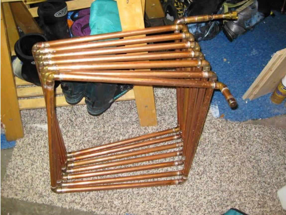
Copper part of heat exchanger
