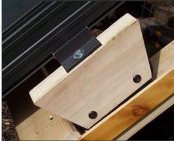
The Flush Mount (AE-FM) brackets are designed for direct roof mounting and provide about 3-4 inches of clearance between the collector back and the roof surface so that leaves and such can slide down the roof surface and not get jammed up under the panel. These are the mounts we used for our AE-40 collectors.
