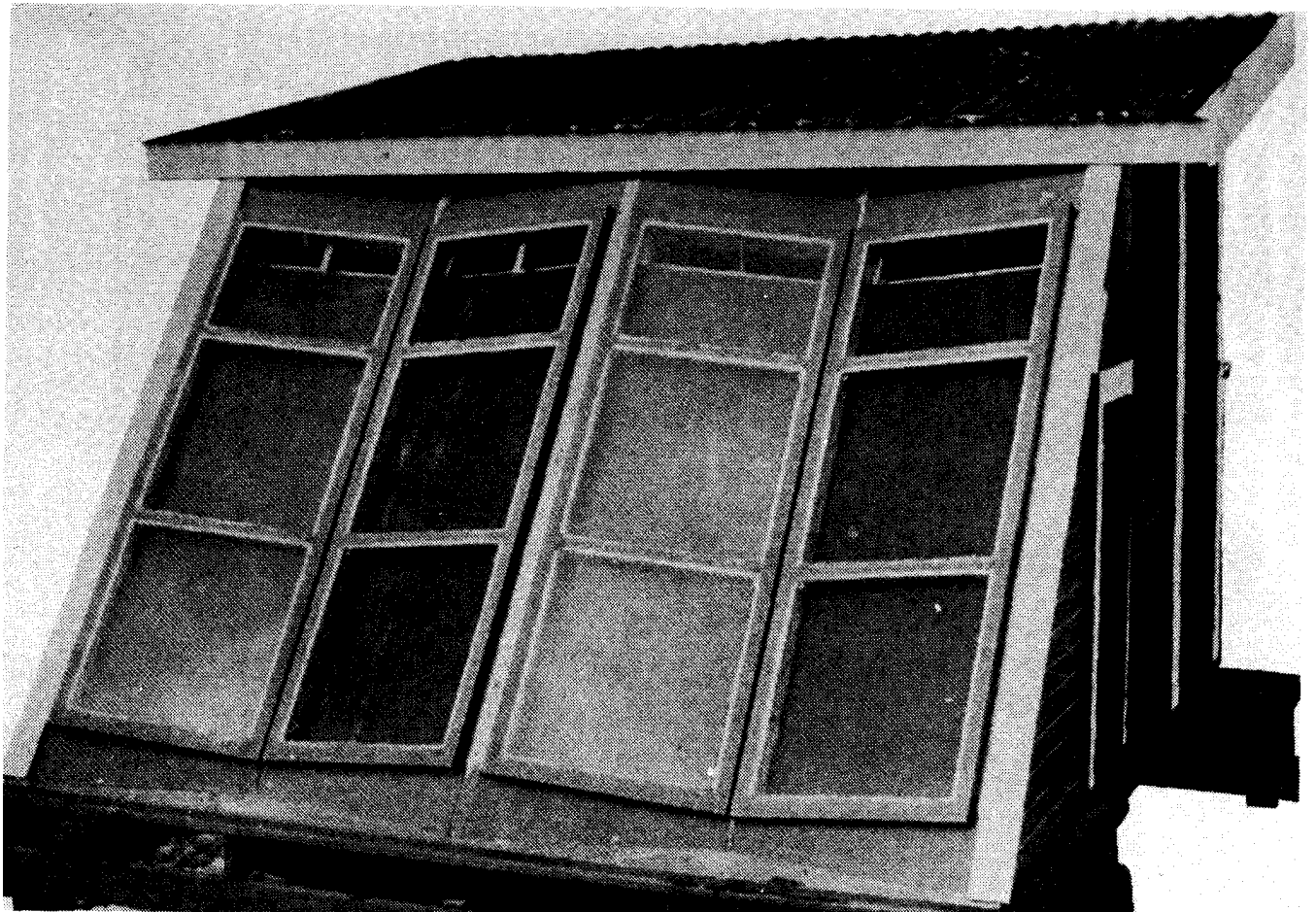
Figure 1. --South side of lumber dryer showing slightly rotated solar-heat collector units at 40° angle from the vertical. Each heat collector unit has a window glass sash mounted on it. The heat-collector unit consists of black sheet metal fastened above a hard board back. Termination of heat collector unit near top of sash allows flow of warm air from within heat collector into dryer proper.
