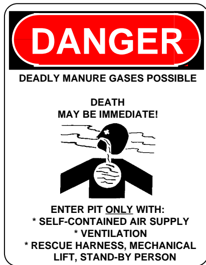
Figure 4. Example of a warning sign placed outside an anaerobic digester.
