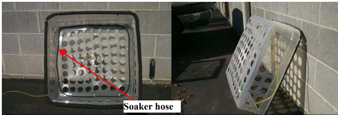
Figure 1. Return Basket Hood, front and side views
