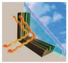
**Cold-Climate Windows Keep Heat In**Double-pane windows with low-e coating on the glass reflect heat back into the room during the winter months.
