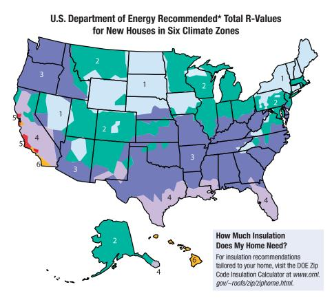
\* These recommendations are cost-effective levels of insulation based on the best available information on local fuel and materials costs and weather conditions. Consequently, the levels may differ from current local building codes. In addition, the apparent fragmentation of the recommendations is an artifact of these data and should not be considered absolute minimum requirements.
