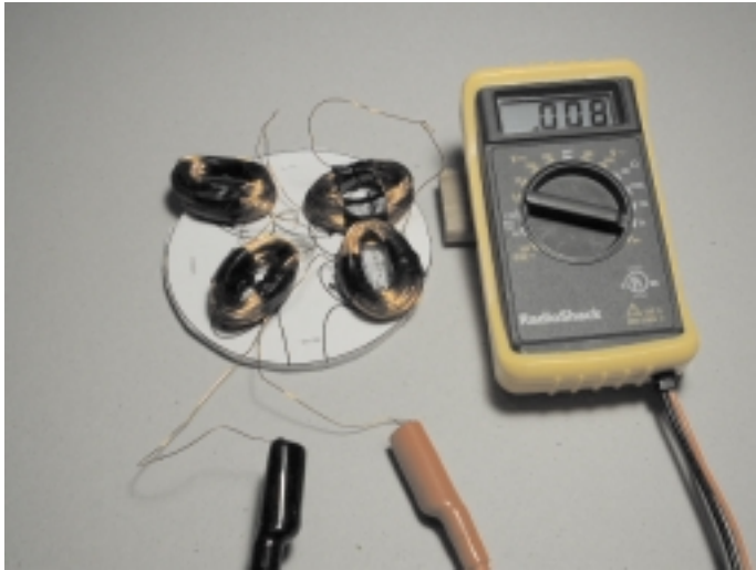
Check to make sure you have good connections between the coils. The Pembina Institute
