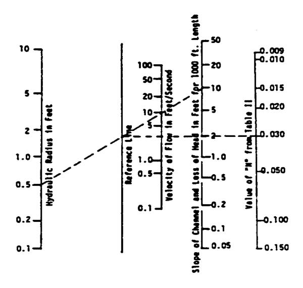
However, a smaller channel can be built by sacrificing some water head. For example, you could build a channel with a hydraulic radius of 0.5 feet or 6 inches. To determine the amount of head that will be lost, draw a straight line from the value of "n" through the flow velocity of 4 [feet.sup.3]/second to the reference line. Now draw a straight line from the hydraulic radius scale of 0.5 feet through the point on the reference
