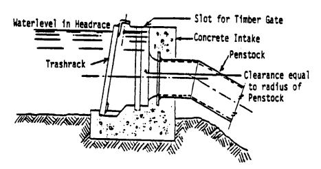
SECTIONAL ELEVATION: INTAKE TO PENSTOCK OF SMALL WATER TURBINE
