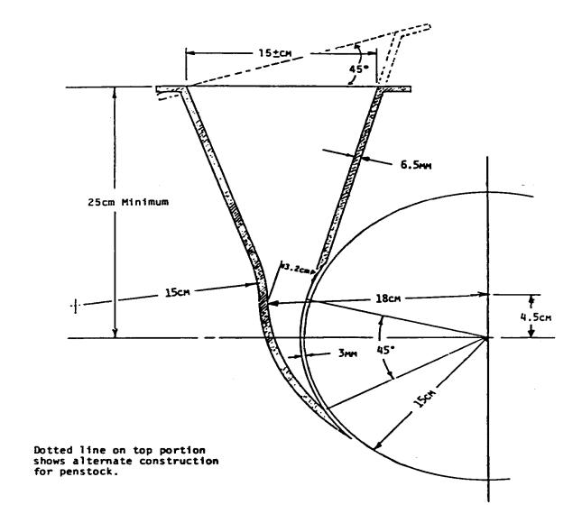
Figure 19. Details of Michell Nozzle
