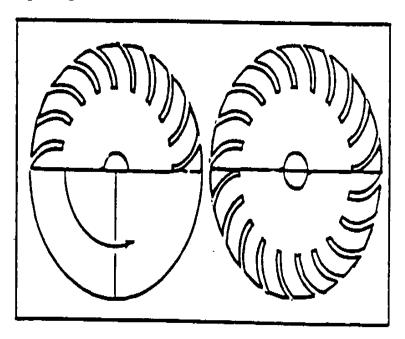
Figure 7. Bucket Slots on Template
