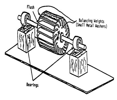
Figure 17. Turbine in Balance
