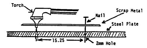
Figure 10. Cutting the End Plates
