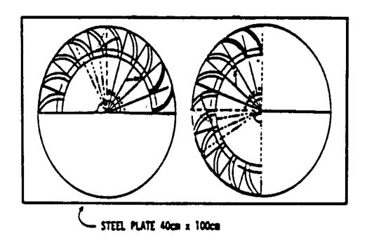
Figure 5. Trace Template on Steel Plate
