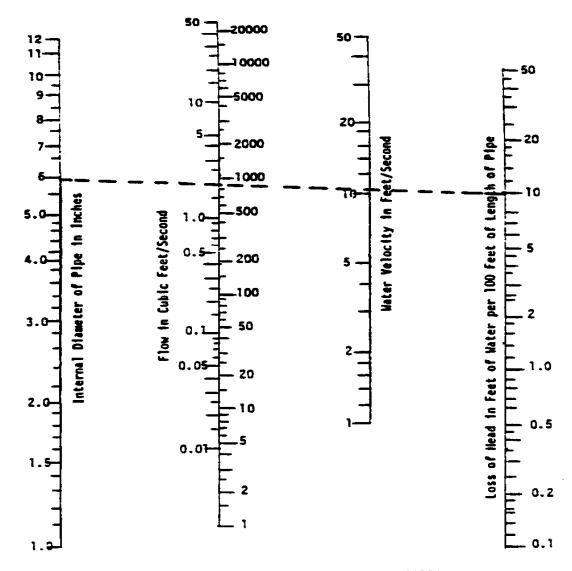
NOMOGRAPH FOR HEAD LOSS IN STEEL PIPES
