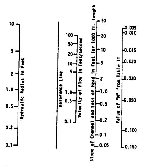
Fall of Channel (or Slope) in feet per 1000 feet of Channel Length (The total fall is equal to the Loss of Head in Feet through the Channel)
