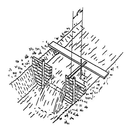
Measure the depth of the water above the bottom edge of the weir with the help of a stick on which a scale has been marked. Determine the flow from Table 1 on page 56.
