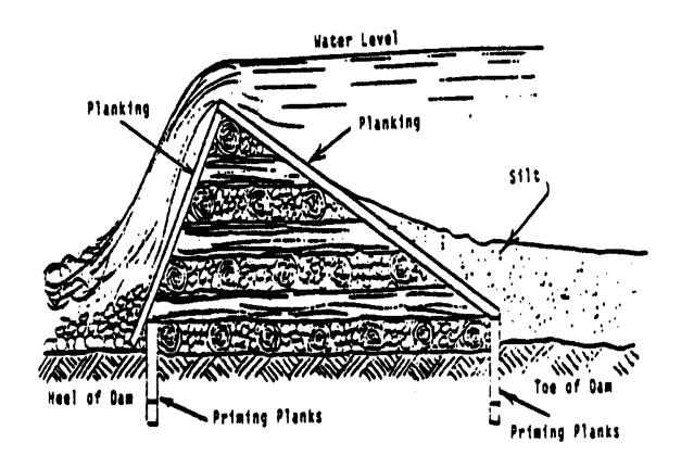
Crib Dam with Downstream Planking
