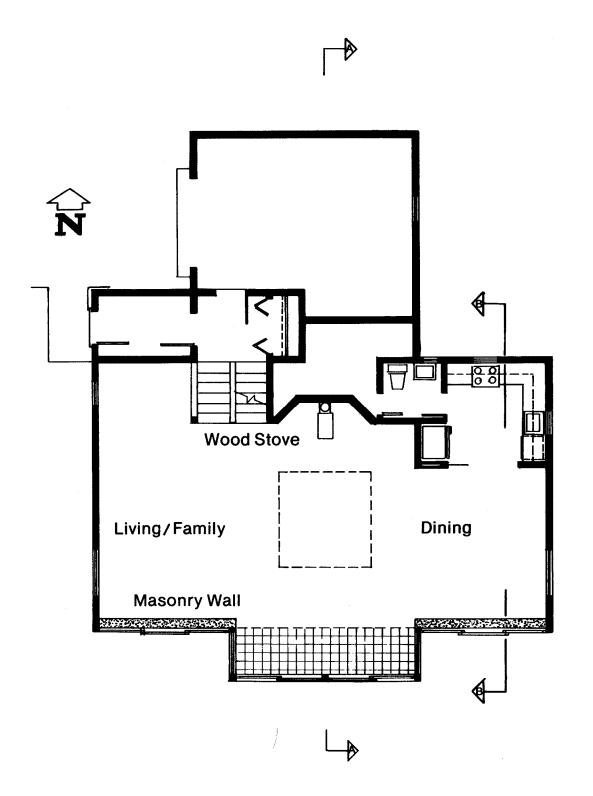
an air-lock entry. The house is carefully caulked and weather stripped; walls and roof are insulated with fiberglass batting (R23,30).
