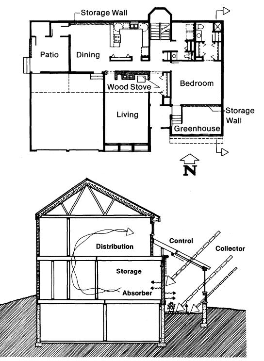
of the roof. The heat is **absorbed** and **stored** in the dining room masonry wall and floor, and in another masonry wall that separates the living room and kitchen on the first story, and a bedroom and balcony on the second story. This wall is also charged with heat from the living room wood stove. On fall and winter evenings, stored heat is **distributed** as it radiates into living and sleeping areas on both levels.
