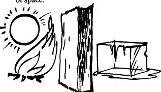
Glazing Layers of glass or plastic, used in windows and other solar devices for admitting light and trapping heat.
