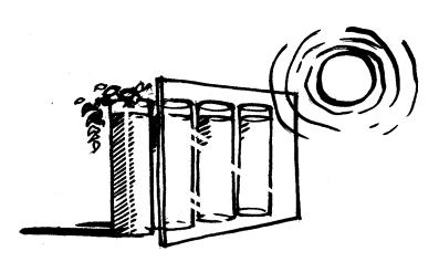
Another type of solar wall substitutes water for masonry. Tall cylinders of water, 55-gallon barrels, and specially-fabricated water walls are common. The water containers radiate their solar heat directly to the room. These walls are often referred to as "thermal storage walls."
