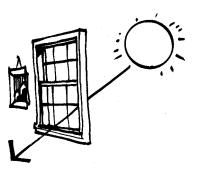
furniture store the excess heat. Movable insulation can cover the windows at night to reduce heat loss. South glass takes advantage of the winter sun's low position in the sky. In the summer, when the sun is high, the glass is easily shaded by roof overhangs or trees. Solar windows are often referred to as "direct gain" systems.
