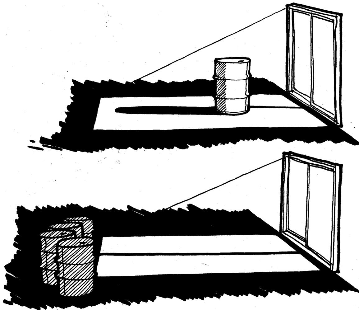
The temperature swings of thermal mass placed in direct sunlight will be about twice the temperature swings of the room itself. Mass shaded from the sun inside the room (such as in north walls) will fluctuate in temperature about half as much as the room. Thus, solar radiated mass stores four times more energy than the shaded mass.
