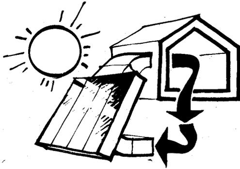
roughly 200 square feet can achieve the 25 percent figure for a well-insulated 1500-square-foot house in a cold climate. Half as much area is needed in a mild climate.
