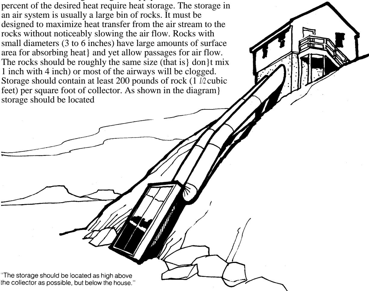
"The storage should be located as high above the collector as possible, but below the house."
