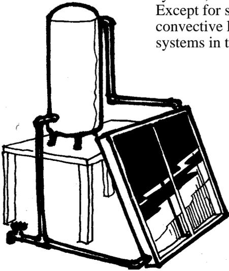
Variations on the design are used to heat water for domestic purposes. Hundreds of thousands of pumpless, "thermosiphoning" (heat convecting) solar water heaters have been used for decades. In fact, convective loop water heaters were patented in 1909. By 1918, 4,000 such water heaters were in operation in Southern California.
