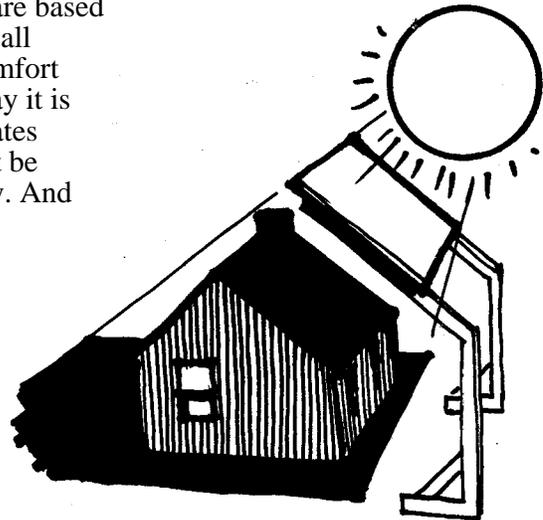
By far the first and most important step in cooling is to keep sunlight from falling on your house, so first we'll discuss "solar control." We'll also discuss natural cooling by ventilation, evaporation, sky radiation, and nesting of buildings into the earth.
