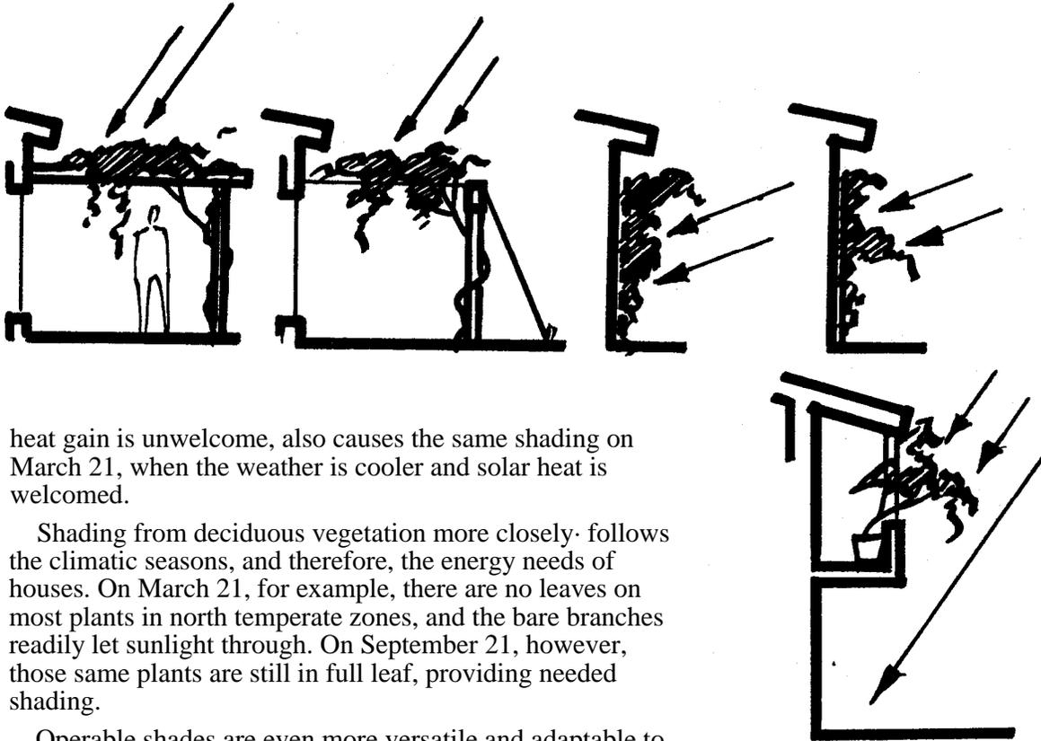
heat gain is unwelcome, also causes the same shading on March 21, when the weather is cooler and solar heat is welcomed.
