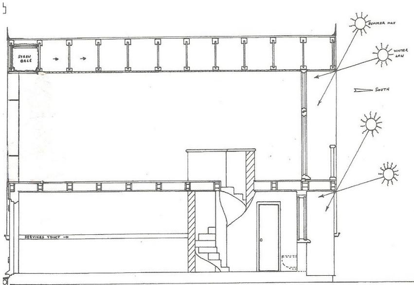
Sectional side elevation is to show how to control the mid-winter & mid-summer Sun penetration by recessing the glazing both to the balcony and the ground floor.
