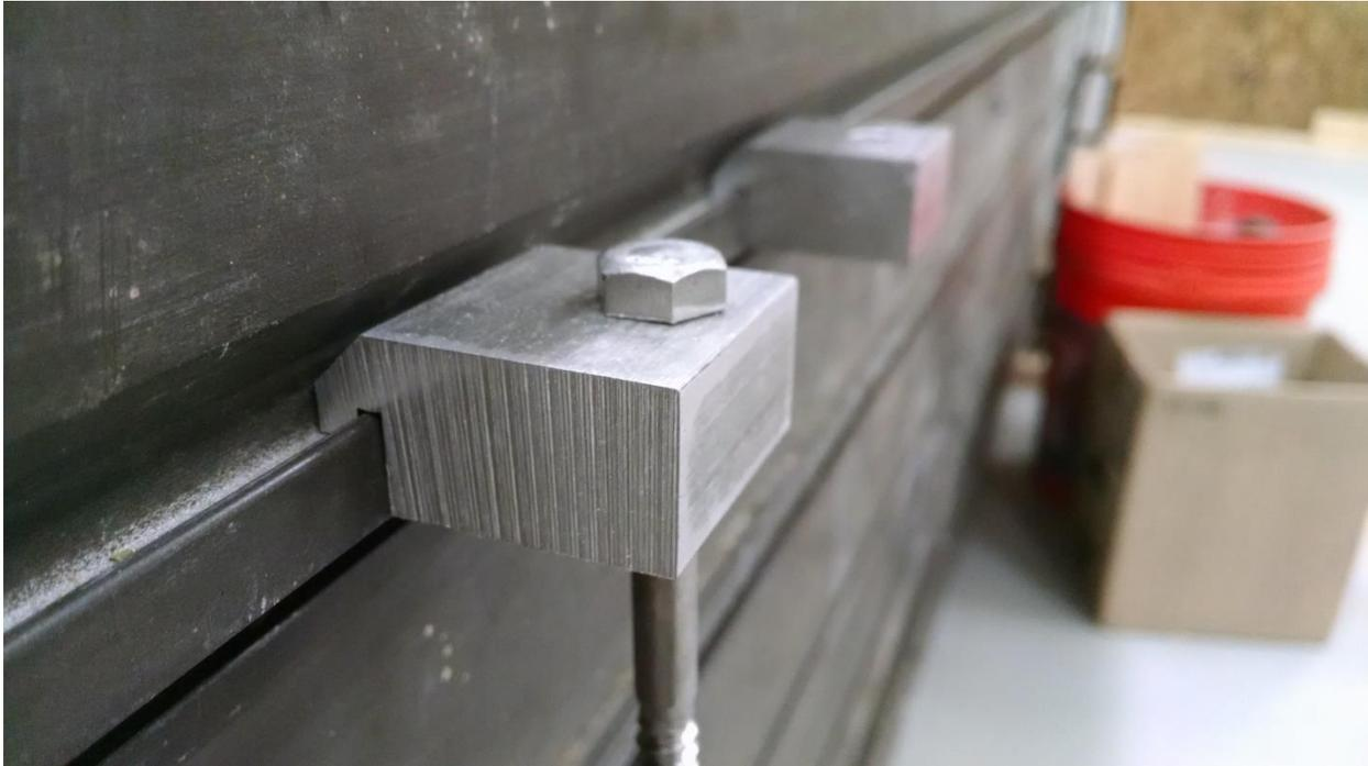
Custom made mounting brackets with a stainless-steel lag screw.
