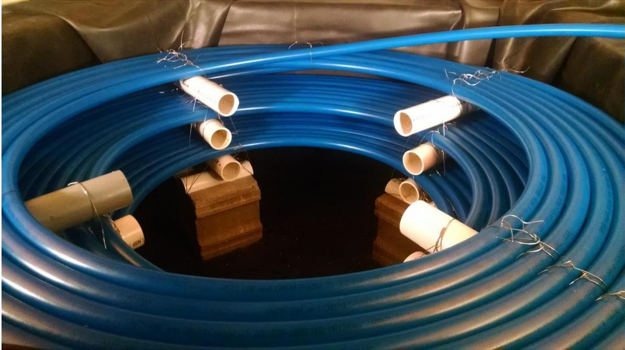
Finished Heat Exchanger coil.
