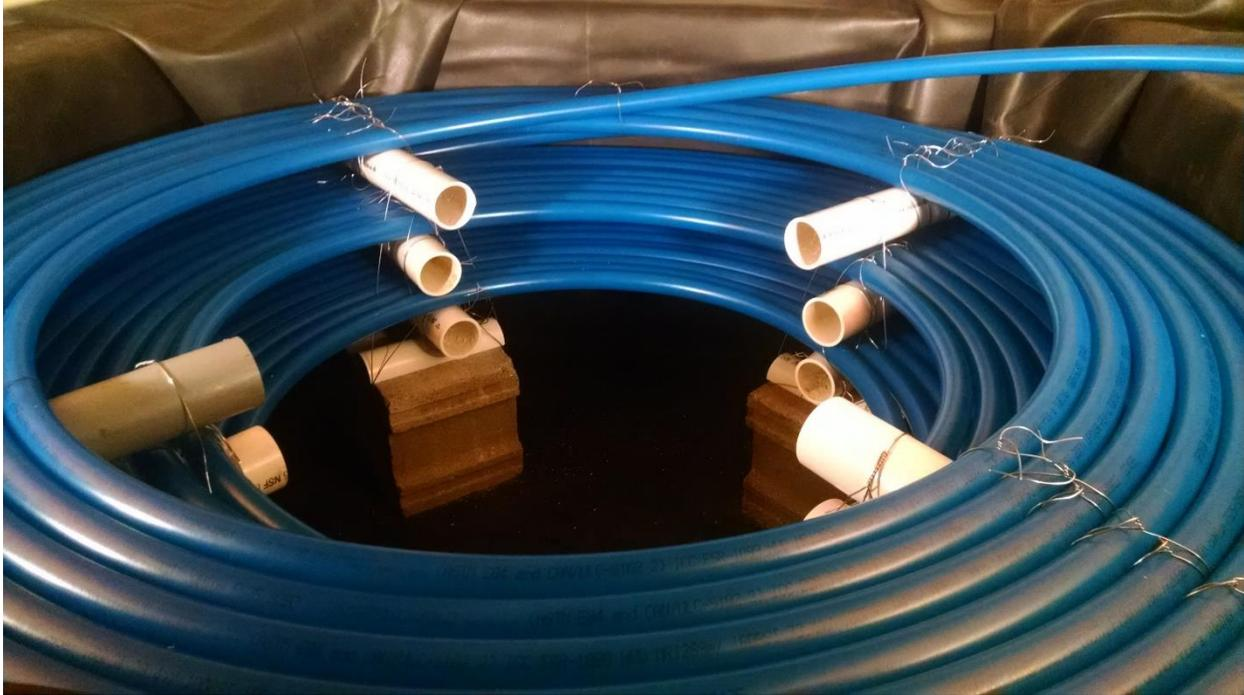
Finished Heat Exchanger coil.
