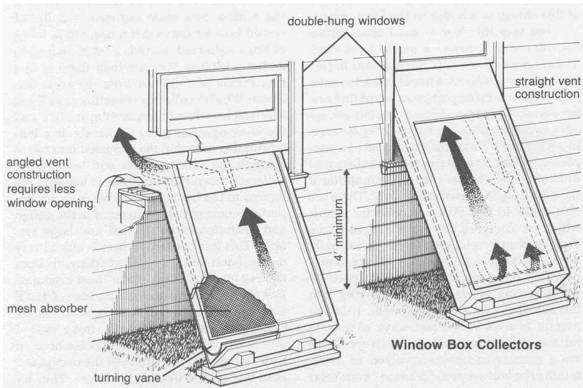
Figure 2-1: *Above* and on opposite page. Window box collectors and TAPs are easy-to-build collectors that deliver their heat by natural convection. They are best used to heat rooms that are frequently occupied and that require daytime heating. Window box collectors are self-damping at night. TAPs require lightweight backdraft dampers to prevent reverse thermo siphoning when the sun isn't shining.
