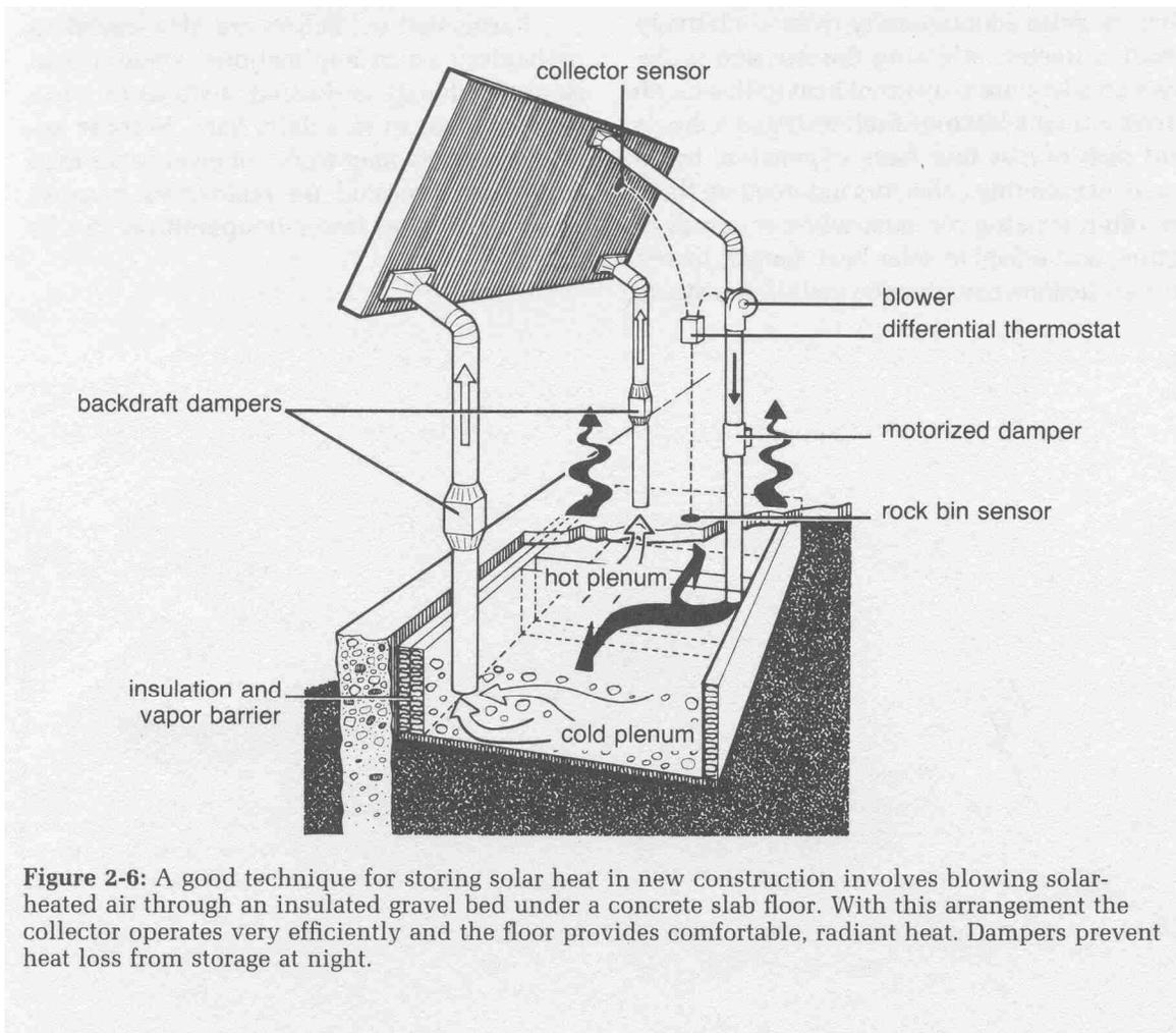
**Figure 2-6:** A good technique for storing solar heat in new construction involves blowing solar-heated air through an insulated gravel bed under a concrete slab floor. With this arrangement the collector operates very efficiently and the floor provides comfortable, radiant heat. Dampers prevent heat loss from storage at night.
