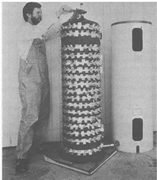
**Photo 2-2:** Tank-type exchangers for heating water are easy to build and install in active solar air systems. Shown here is a 50-gallon finned exchanger, which will be used for summer water preheating in a small two-mode system.
