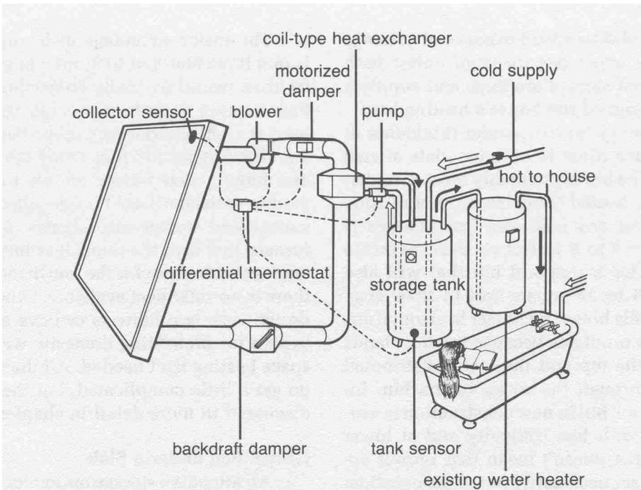
**Figure 2-4:** An air-to-water heat exchanger is required for heating domestic water with a solar air collector. A coil-type heat exchanger can be mounted inside a duct to take heat from solar air. Heated water is then circulated by a pump to a storage tank. Or a tank-type heat exchanger can transfer heat by blowing solar air directly over and around the storage tank.
