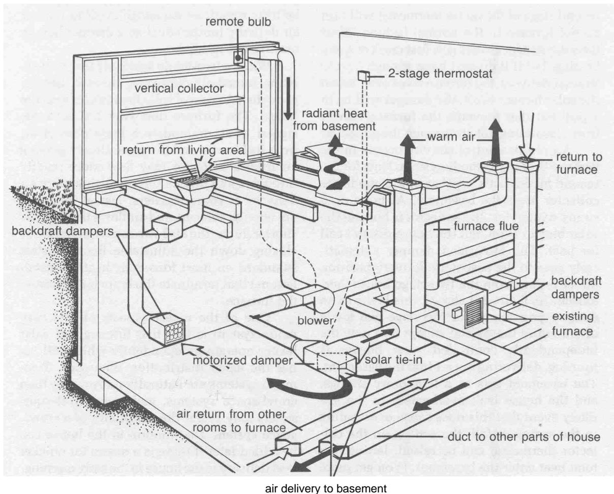
**Figure 2-3:** This two-mode system is simpler than it first appears. When the upper floor calls for heat and the collector is on, solar air is blown into the existing ductwork to warm the living area. When the needs of the upper floor have been satisfied, the motorized damper changes positions, and solar heat is delivered into the basement and stored in the concrete walls there. Note that two returns (inlets) to the collector, each with a backdraft damper, are required in this system.
