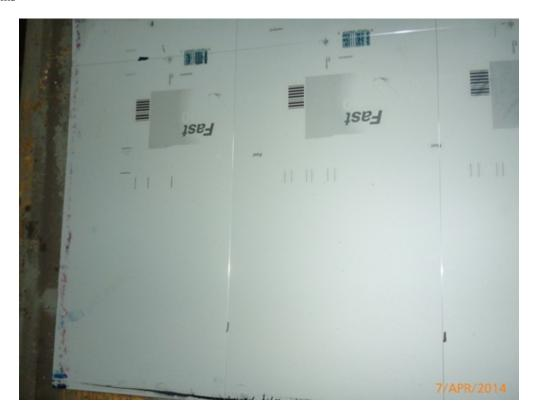
Place the plate over a table edge bend it up and down 2-3 times and it will separate clean.
