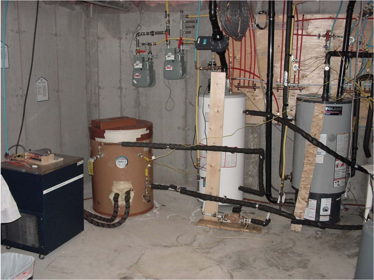
Figure 3: DWHR test setup
