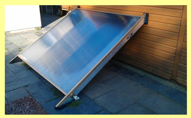
The polycarbonate was secured with 25mm aluminium angle iron sprayed gold to give it a bit of bling. Handles were attached to help move it around. It's a heavy beast. Feet were made to spread the weight.
